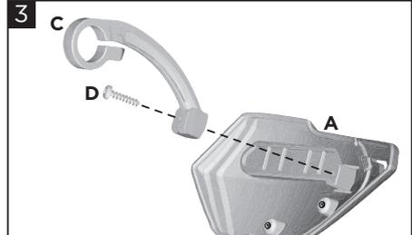
**Tighten the brackets (C) to the cover (A) using the screws (D).**
