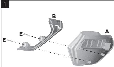
**Tighten the spoiler (B) to the cover (A) using the screws (E).**
